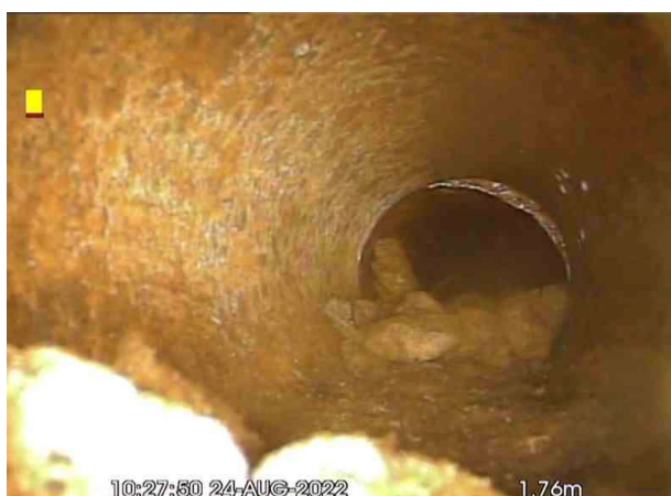
DX_6d1db3e8-1221-425a-87dd-3074f4980fe4_20220831_141 526_375.jpg, 00:00:18, 1.76 m Settled deposits, coarse, 45% cross-sectional area loss
