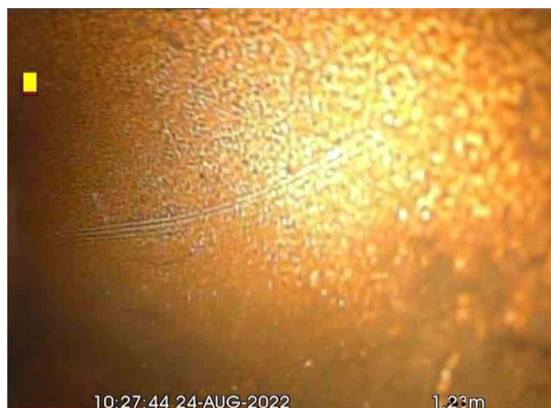
DX_79a51984-81b6-45de-8f5e-51a679451a55_20220831_14 1412_997.jpg, 00:00:12, 1.23 m Line deviates left
