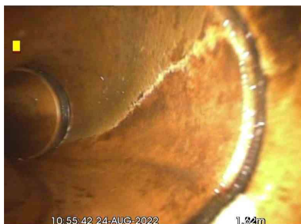
BX_ab3ec797-15f8-4b2c-a4aa-2d8e63d9aa1f_20220826_144 059_050.jpg, 00:00:11, 1.62 m Line deviates left
