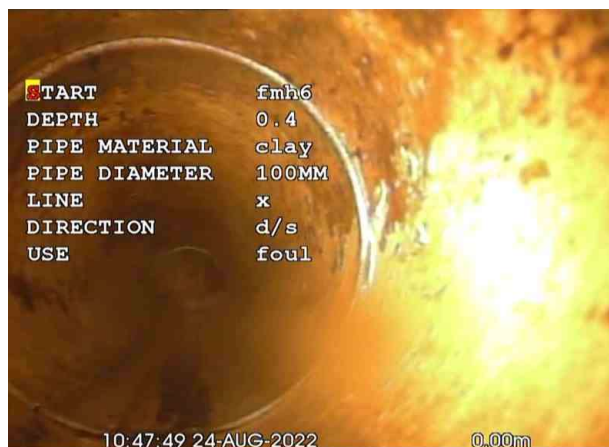
FMH6X_2ec624e6-e24b-4904-9b5f-b8d1b2ea1bba_20220831_084218_366.jpg, 00:00:00, 0.00 m Start node, manhole, reference: FMH6
