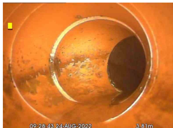
FMH1X_65d60478-abd0-40c1-84bb-baf347cda3a2_20220826_105030_744.jpg, 00:00:16, 3.81 m Line deviates right
