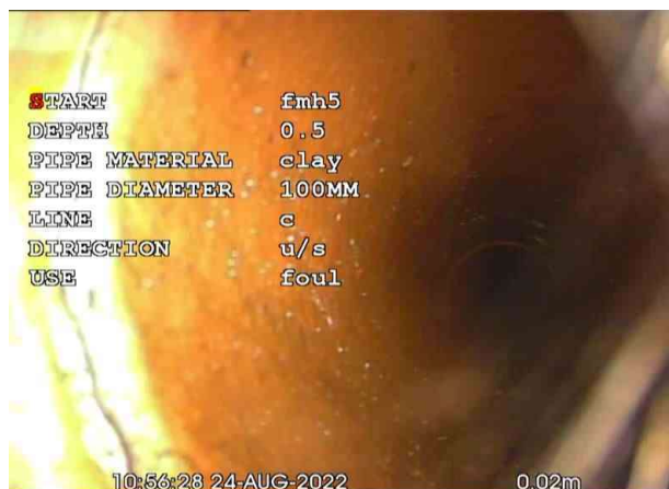
CX_3d61e0a4-39d0-40e5-8c0e-54ffa6ad66d5_20220830_120 523_840.jpg, 00:00:00, 0.00 m Start node, manhole, reference: FMH5
